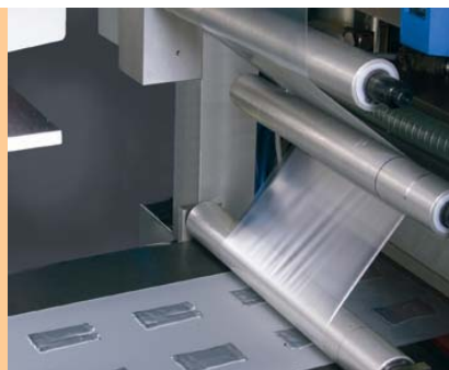
Lamination of a lidding foil via the freshly dosed gel
