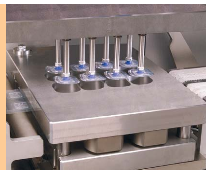
Pick-and-place transfer of the patches onto the vacuum transfer belt to the bag packaging station
