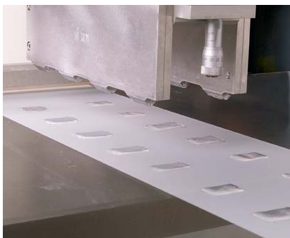
Dosing heads for application of the active gel substance onto the carrier foil
